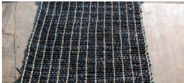
Textile hydraulic barriers for the enhancement of polishing ponds (containing floatable elements and weights for stabilization)
