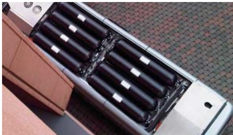
Figure 3.3: Hydrogen tanks mounted on RVK's APTS-Phileas fuel cell bus (350 bar, Type 3 tank with aluminium liner, 8 x 205 litre) (source: Dynetek Europe GmbH)
