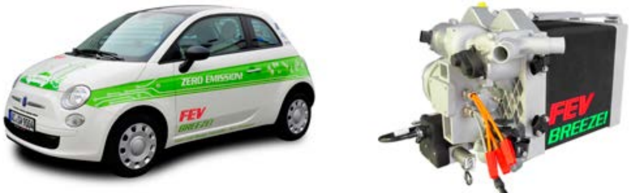
Figure 4.13: Experimental vehicle from the FEV Liiona fleet (SmartWheels project) and conceptual packaging of the BREEZE! range-extender module (source: VKA RWTH Aachen)
