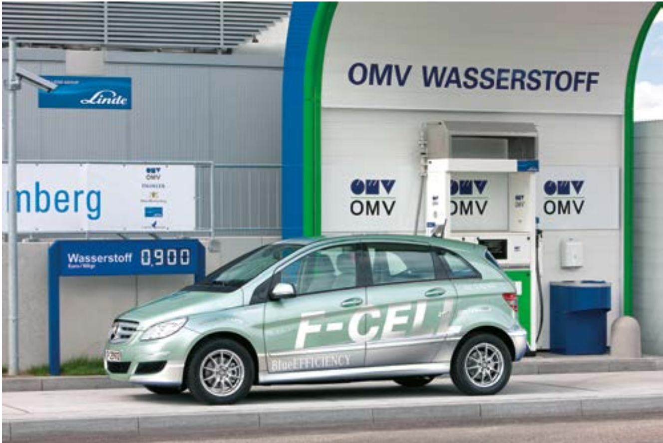
Figure 4.8: The Mercedes-Benz B Class F-CELL (80 kW PEM fuel cell, 100 kW electrical propulsion, Li ion battery for 30 kW output, range approx. 400 km, pressurised-hydrogen storage [700 bar], consumption 103 MJ/100 km or 2.9 l diesel equivalent per 100 km) (source: Daimler AG)
