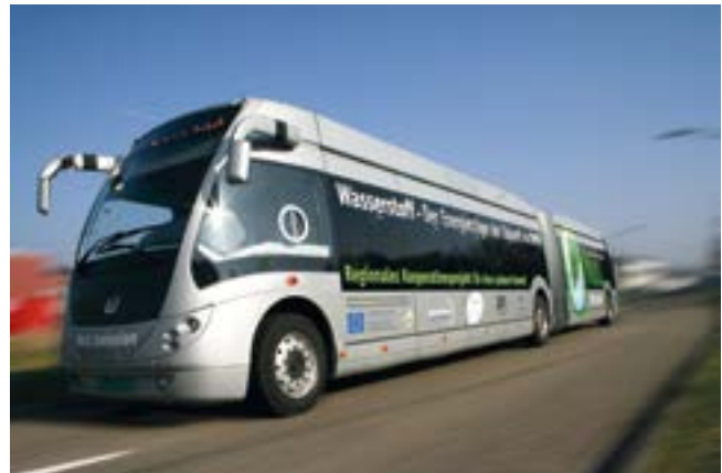
Figure 4.12: “Phileas” fuel cell articulated bus operated by Regionalverkehr Köln GmbH (source: RVK)
