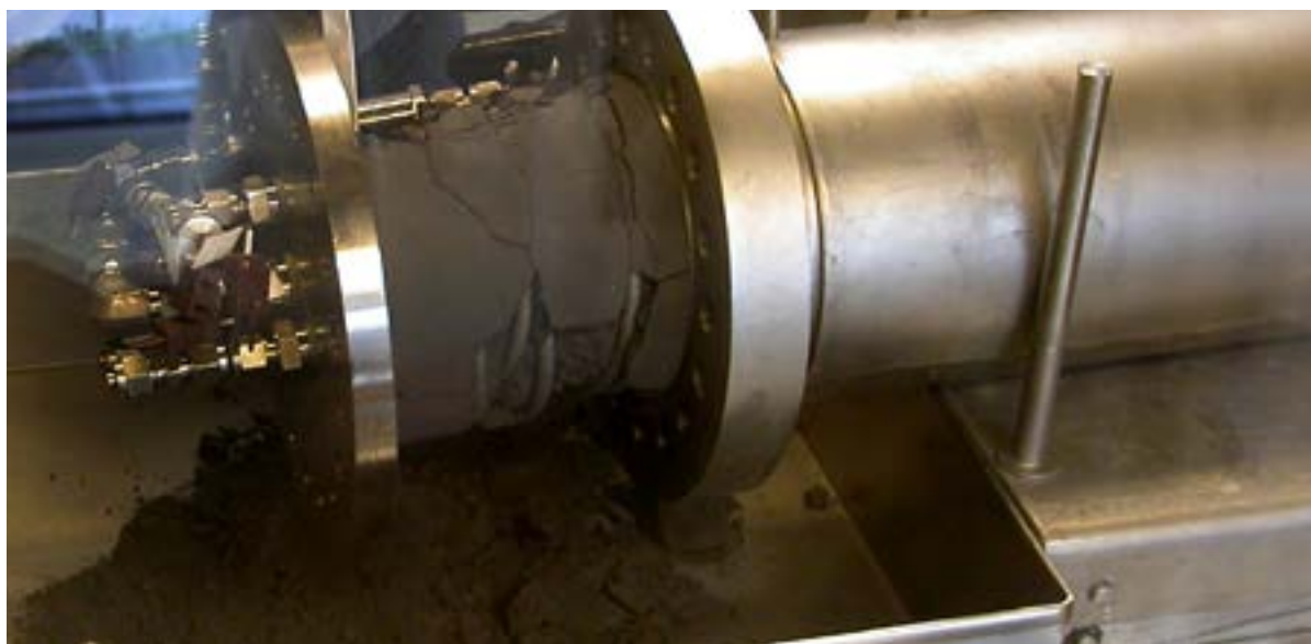
Figure 3.5: Example of a storage tank functioning as an H 2 source for an HT PEM fuel cell (Note: opened storage tank for 3 kg NaAlH 4 ; construction and development as part of AiF project 247ZN, co-operation partners: MPI Mülheim, ZBT Duisburg, IUTA Duisburg)
