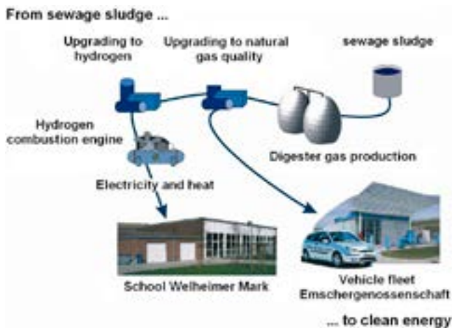
Figure 2.9: System components: "EuWaK – Natural gas and hydrogen from wastewater treatment plants" at the Bottrop wastewater treatment facility (source: EuWaK)
